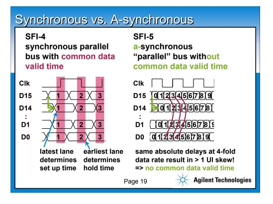
As each channel can independently wander by more than a single period, the word relationship of the parallel is lost through multiplexing and de-multiplexing.
