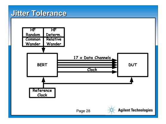
Jitter tolerance can be considered as being the generation of a test signal with a calibrated amount of jitter, and the measurement of the relative or absolute Bit Error Rate performance of a Device.
