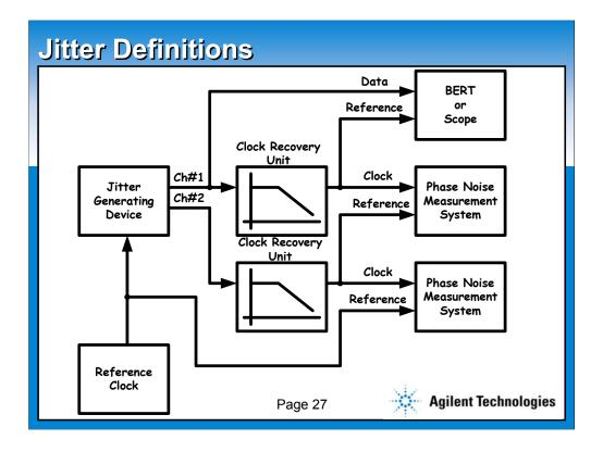
In exactly the same way that jitter is defined by the ITU, the OIF defined different types of jitter that must be measured and tested for the SFI-5 interface.
