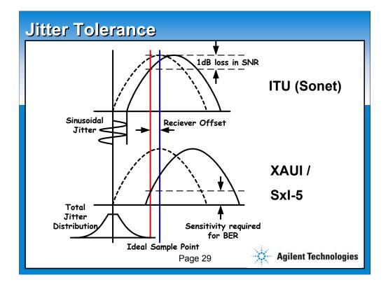
ITU defines Jitter Tolerance for OC-192 or OC-768 in terms of a 1dB relative sensitivity loss for a given sinusoidal time jitter.
