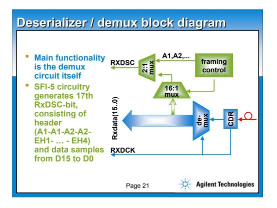
The DSC channel is easily generated by multiplexing the 16 channels together with the framing information.
