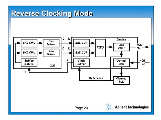
The jitter present on the SFI-5 signals is a function of the clocking mode of the 40G SerDes.
