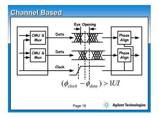
As the baud rate increases it becomes impossible to control the relationship between the data channel, and a Channel Based interface must be adopted i.e. SFI-5.
