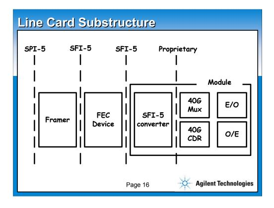
A typical 40G Line Card solution consists of a Framer / FEC chip set directly on the line card, and a plug-in module solution.
