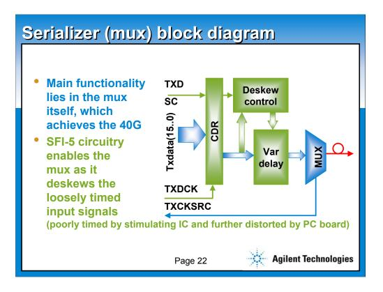
De-skew is performed by a control block which monitors the DSC channel and controls the delay of each channel.
