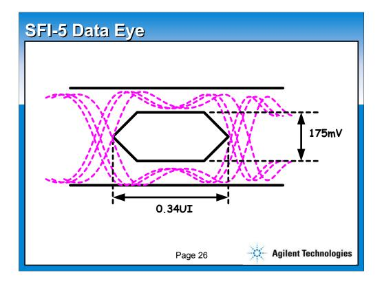
SFI-5 defines the electrical signalling for the data as a differential receive data eye, with a given eye opening. When DC coupled the common mode at the transmitter and receiver must in addition lie with defined limits.
