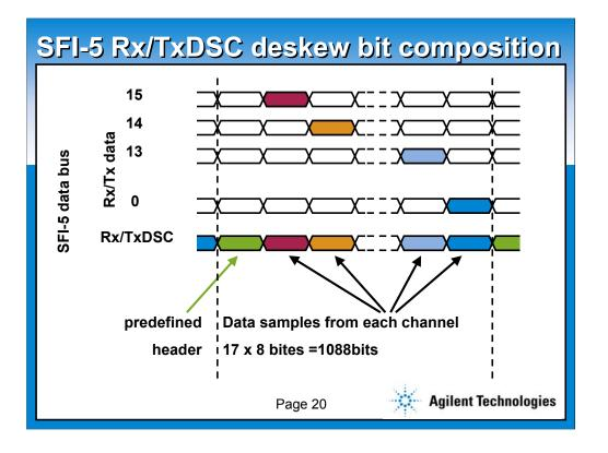
De-skewing is achieved by the 17<sup>th</sup> bit (TXDSC or RXDSC), which contains data samples from each of the 16 data channels, each 8 bytes long, in a round robin fashion following after an 8 byte header.
